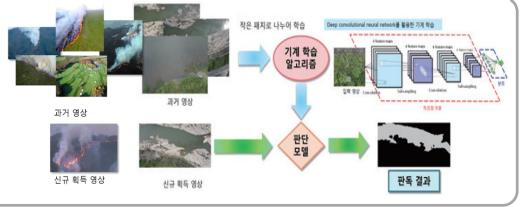
Real-time video acquisition from unmanned aerial vehicles with hybrid power sources for fuel cells and batteries is analyzed based on deep learning to monitor disasters such as fires, landslides, and floods.
