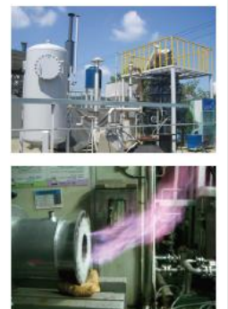
[Figure] CHP System Using Rice Husk Gasifier Combined with IC Engine System in RPC
