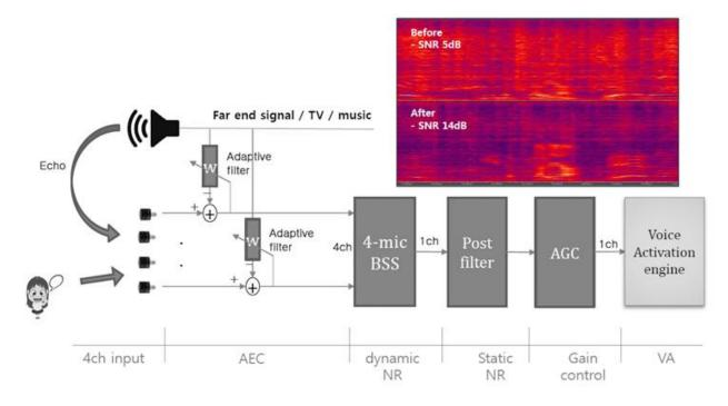
Real-time noise cancelling & auto-gain correction algorithm through multi-channel BSS(Blind Source Separation) engine
