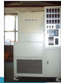
1999-2001 5kW system with NG reformer
